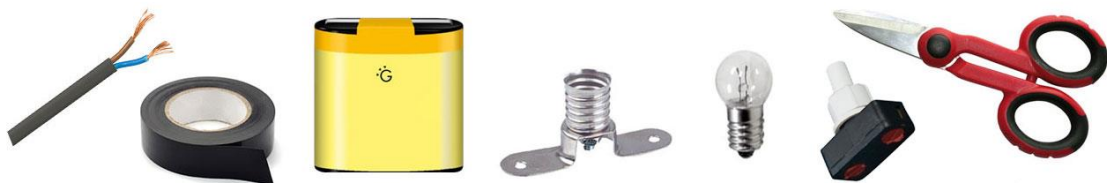
Picture 11 Set of material to build circuits. These batteries are not easy to find anymore, so we used lantern batteries instead
